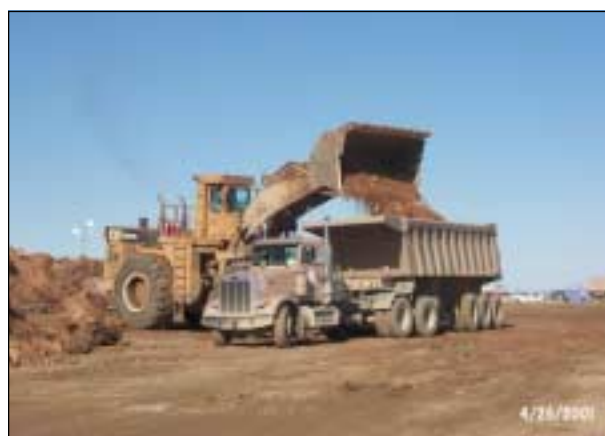
Figure 22. A Caterpillar 992C loader dumping gold ore into a 60-ton truck at True North Mine for transport to Fort Knox Mine mill and transfer directly into the crusher. Photo provided by Kinross Gold Corp.
