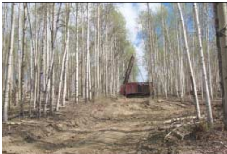
Figure 7. Core drilling at the True North project. Photo provided by Kinross Gold Corp.
