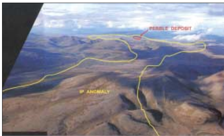
Figure 9. Airborne photo of the Pebble deposit with an outline of a portion of the large induced polarization (IP) anomaly that covers at least six mineralizing centers. The Pebble deposit is outlined in the upper center of the photo. Photo provided by Northern Dynasty Minerals Ltd.
