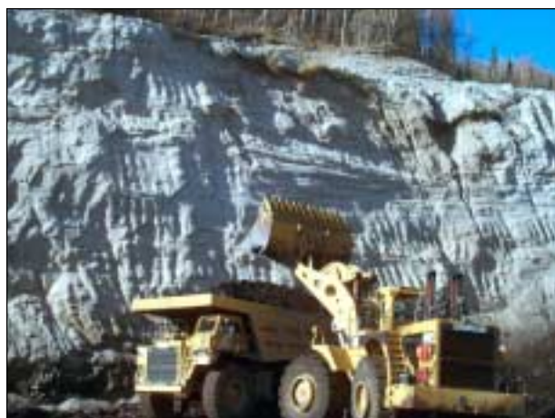
Figure 14. Development at Usibelli Coal Mine Inc.'s Two Bull Ridge pit concentrated on making a box cut down to the coal-bearing seams. A Caterpillar 785 haul truck is being loaded by a Caterpillar 992 loader. Photo by David Szumigala.
