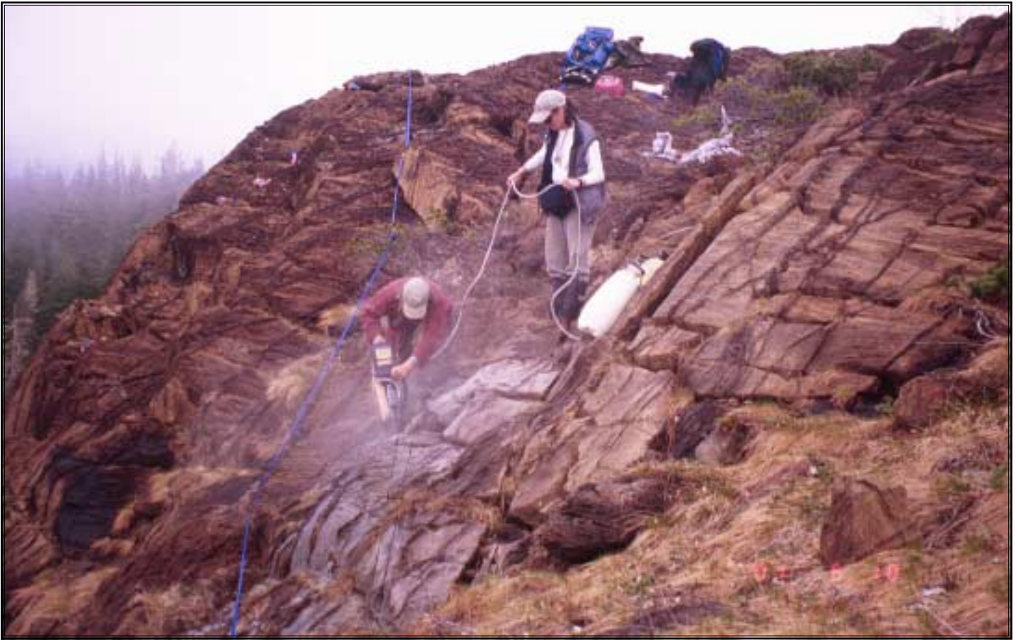
ABOVE: Pete Nyren, assisted by Myriam Figueiredo, using a Partner rock saw to take a channel sample of platinum-group-element-bearing (sample averaged 0.32 ounces per ton platinum + palladium) magnetite stringers in pyroxenite at the North Zone prospect on the Union Bay property, southeastern Alaska. Exploration work conducted by Avalon Development Corp. in 2001 for joint-venture partners Quaterra Resources Inc. and International Freegold Mineral Development Inc. (Photo provided by Avalon Development Corp.)
