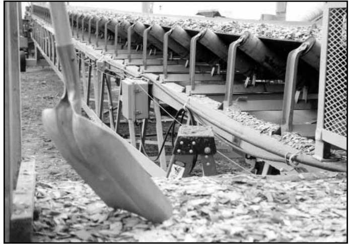
NPI chip conveyor used to load chips. Photo by Dean Brown.
