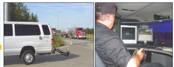
INFRA RED INSPECTION STATION (IRIS VAN)
