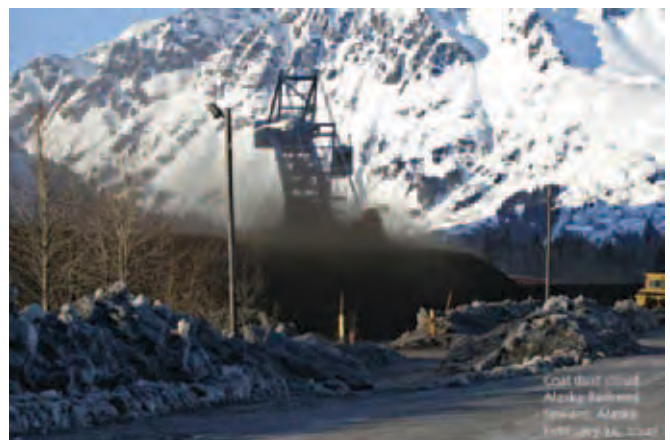
Coal dust produced by loading/unloading operations at the Seward Coal Terminal February 24th 2007.
