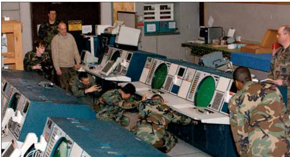
Powering Down. The Alaska Air National Guard's 176th Air Control Squadron (ACS) shut down its old green-and-black-radar-screen Q-93 system that was used to manage air defense operations throughout Alaska. Replacing the old system is the new Battle Control System-Fixed. It's a PC-based, color-monitor system that uses the newest technology to keep track of aircraft in the skies over the state. Photo: Kalei Brooks, DMVA Public Affairs
