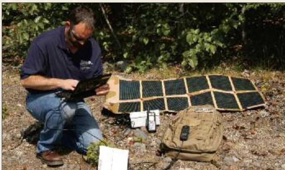
In Contact. Bryan Fisher, operation section chief, DHS&EM, demonstrates how to use these communications back-packs. The packs provide a small team with communications anywhere in Alaska. The easy-to-set-up systems can be powered by an included solar panel, DC or standard 110 AC power. Photo: Jeremy Zidek, DHS&EM Public Affairs
